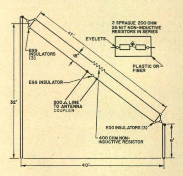
The antenna loads up about the same as any other. However, when adjusting the antenna coupler, try to get maximum loading with maximum capacity in the pi network output
